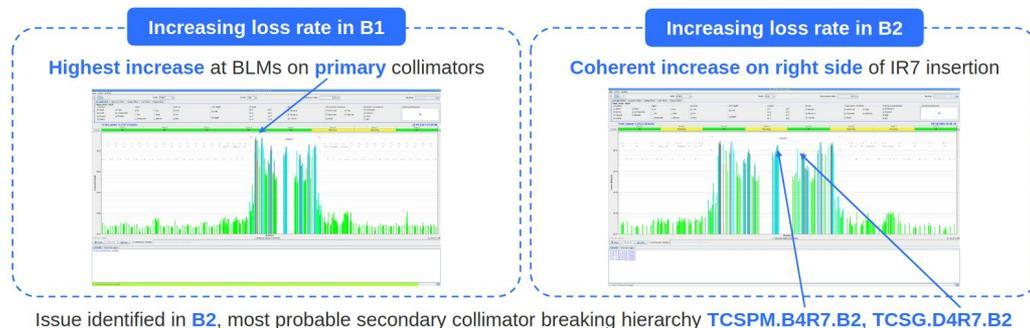
Issue identified in **B2**, most probable secondary collimator breaking hierarchy **TCSPM.B4R7.B2, TCSG.D4R7.B2**
