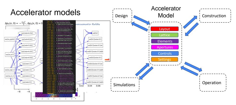
Accelerator physicists and operators inject or extract information into models to design, construct, operate and optimize accelerators.
