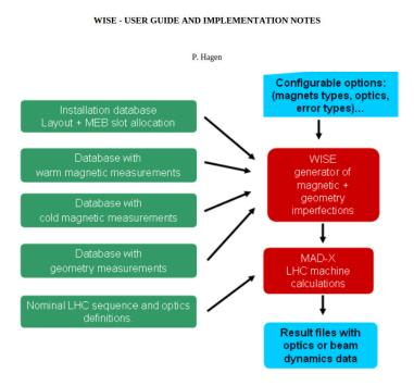
Windows Interface to Simulation of Errors
