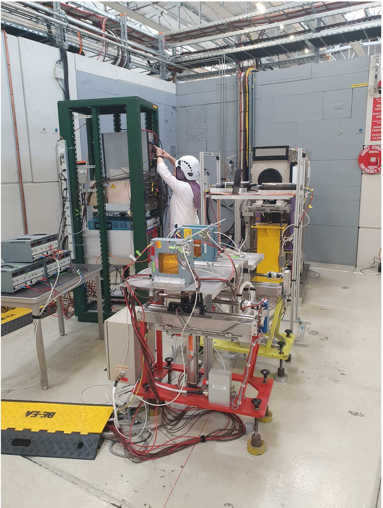
Upstream: XCET and Scintillator of T10, BL4S 2x finger scintillator on stand, XSCA for WENDI (stretch goal, tungsten target on tripod not in picture), BL4S 3x DWC (out of which the first one mimics the "DUT") on XSCA
