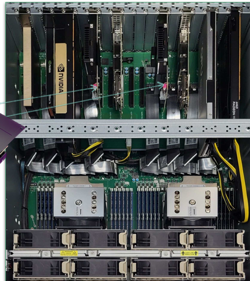
CXL host node at CMS USC. Server supplied by E4 Computer Engineering
