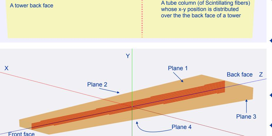
intersection of a line parallel to the z-axis passing through x-y with each of the 4 planes in figure + the front face
