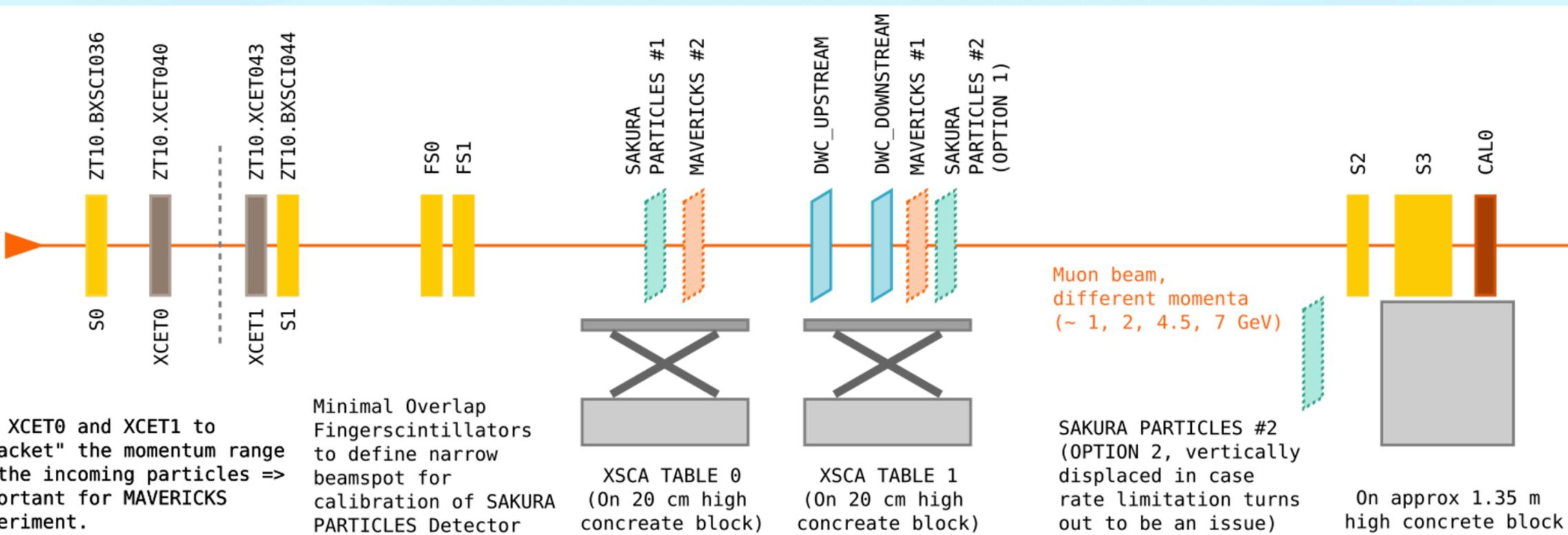
Use XCET0 and XCET1 to "bracket" the momentum range of the incoming particles => Important for MAVERICKS experiment.
