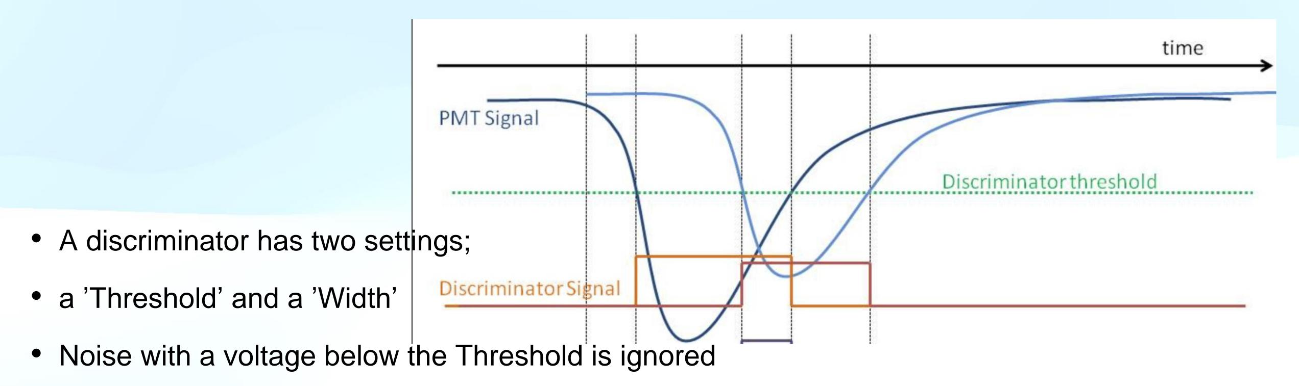
• If the input signal crosses the Threshold, a pulse is generated with the desired Width
