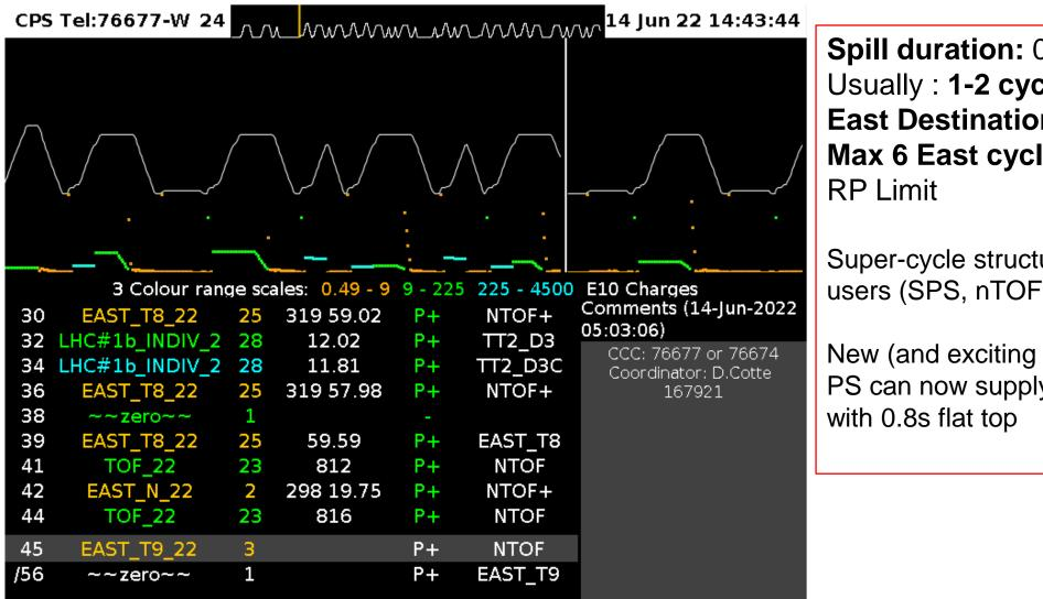
Spill duration: 0.4 second flat top Usually : 1-2 cycles per minute per East Destination Max 6 East cycles / 40 seconds → RP Limit
