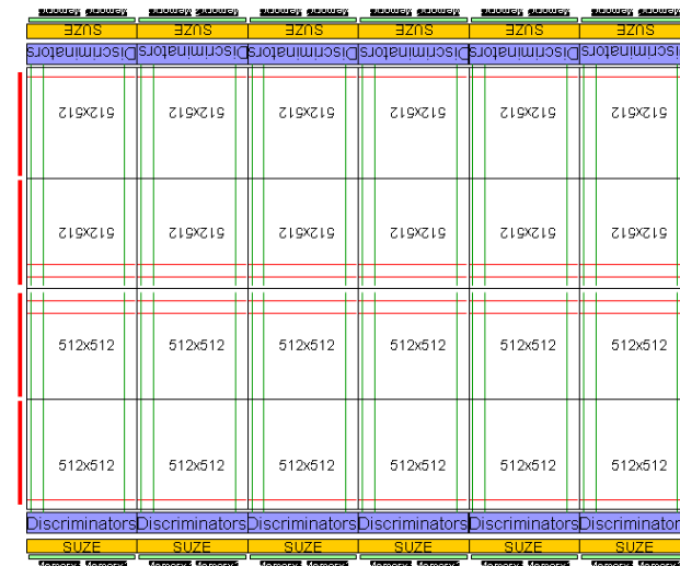
Final sensor \rightarrow \sim 6 \text{ cm} \times 4 \text{ cm} = 24 \text{ cm}^2
