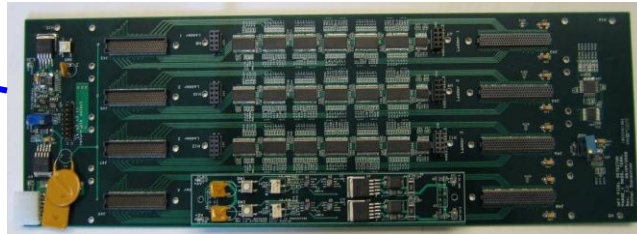
Mass Termination Board + latch-up protected power daughter-card
