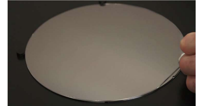
Bonding wave: glass to Si & Si to Si bonding
