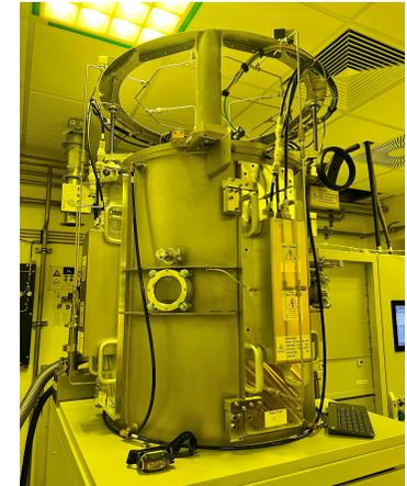
Pulsed DC magnetron vacuum deposition machine
