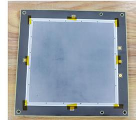
Coating of Germanium for Resistive Anode
