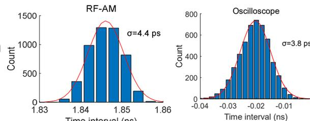
Time jitter of RF Amplifier compared to the oscilloscope
