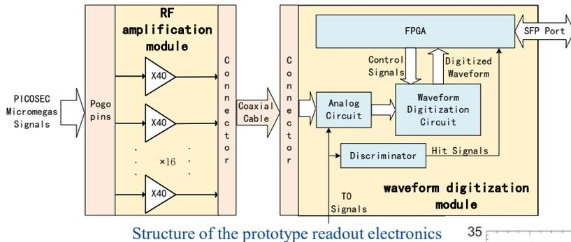
Structure of the prototype readout electronics
