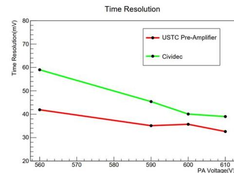
Test beam results for RF Amplifier vs Cividec
