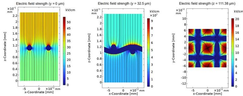
**2. Avalanche development** can be calculated by using microscopic tracking for the electron in Garfield++.
