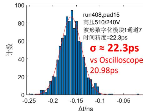
Test beam results for RF Amplifier + drs4 WDM
