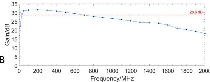
Gain frequency response curve of RF Amplifier
