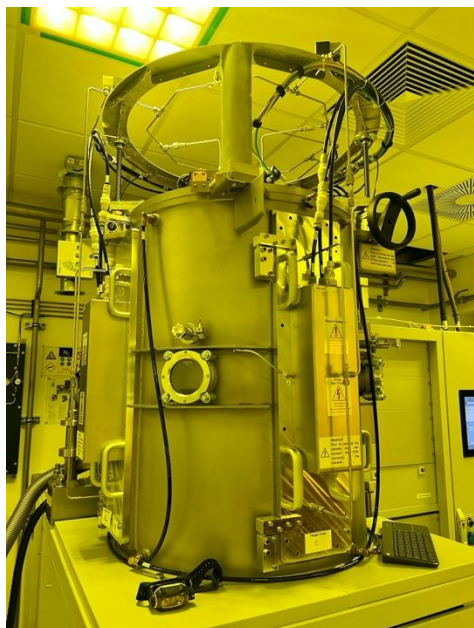
Pulsed DC magnetron vacuum deposition machine
