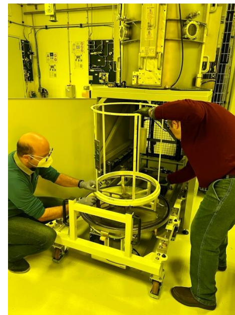
Loading the drum into the chamber
