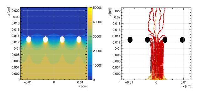
Representation of the electric field inside the Micromegas
