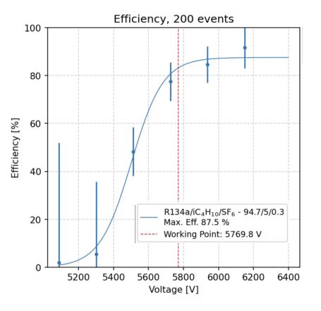
$\begin{array}{ll} \textbf{Sigmoid fit:} \quad \epsilon(HV_{eff}) = \frac{\epsilon_{max}}{1 + e^{\gamma(HV_{eff} - HV_{50})}} \\ \text{Where:} \\ \text{HV}_{eff} \text{: Applied voltage corrected by T/P} \\ \epsilon_{max} \text{: Maximum efficiency} \\ \text{HV}_{50} \text{: Voltage where efficiency} = 50\% \end{array}$
