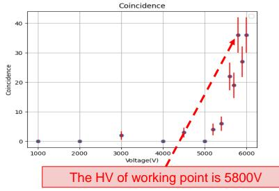
• Number of each trigger chamber for different voltages in 100 sec.
