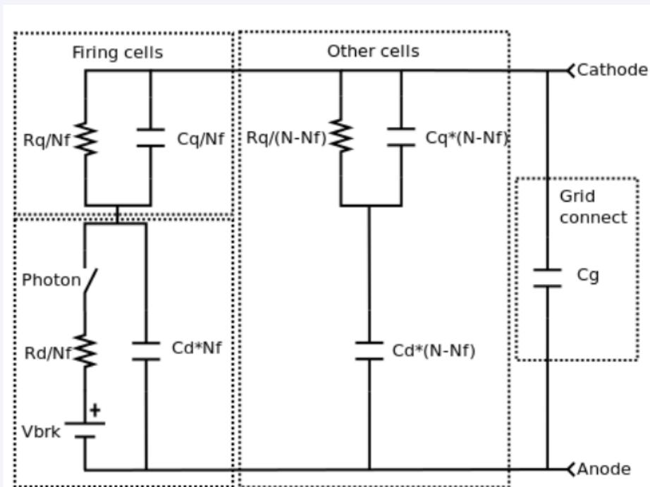
**R<sub>q</sub>** Quenching resistor value
