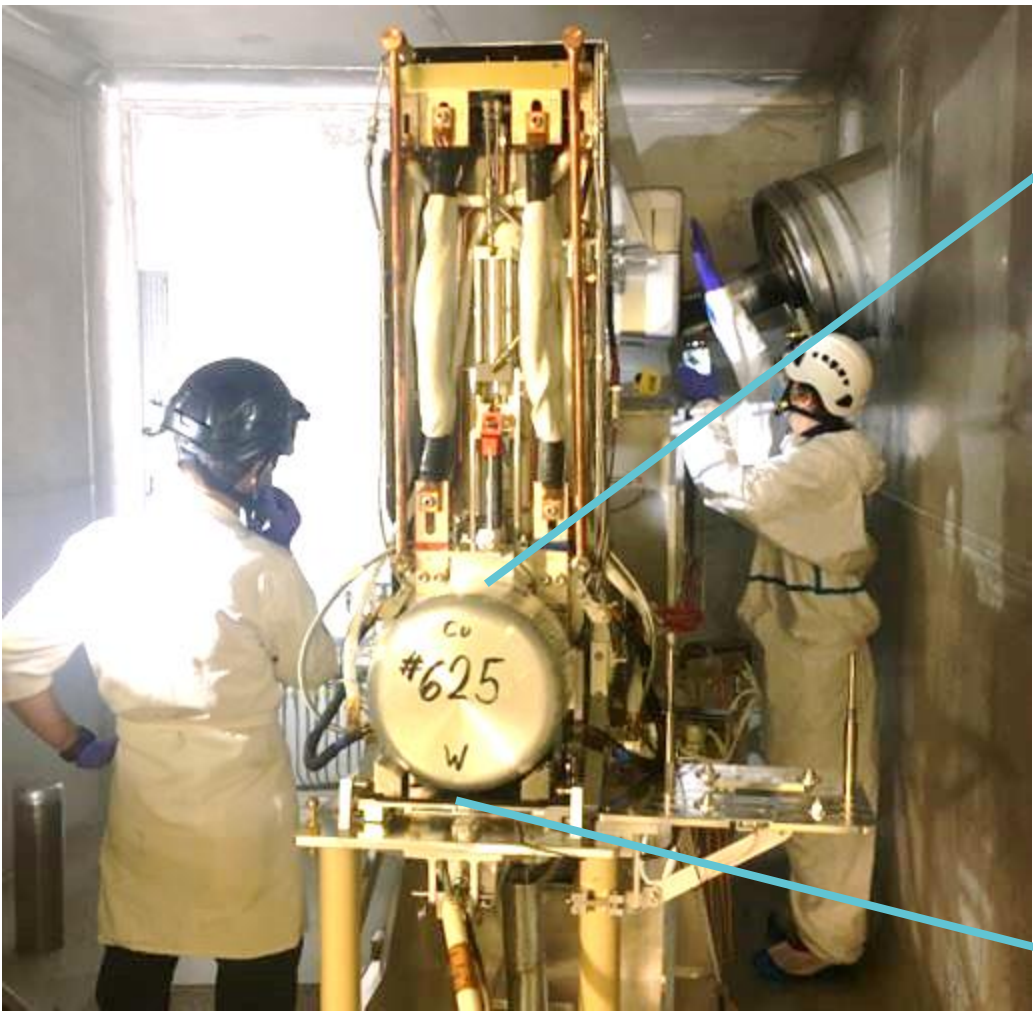
Fig. 1. Target and ion source assembly with plasma ion source MK5. The vacuum valve is part of the assembly.
