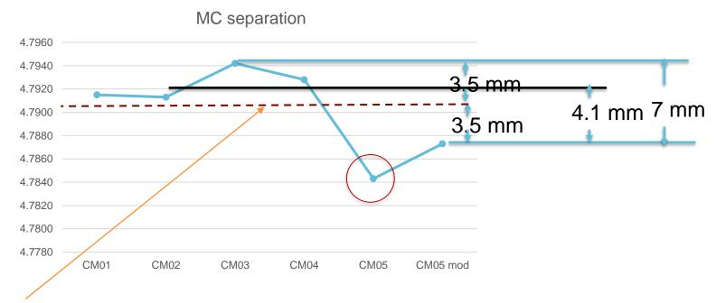
With the new target MCS value the CMS values for all magnets would be within  $\pm 5 \text{ mm}$
