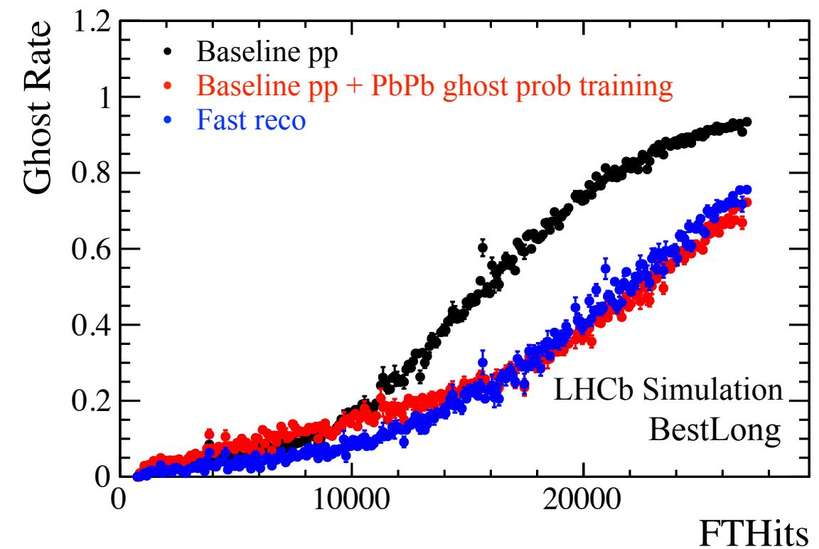
**Significant improvement**  $\rightarrow$  the ghost rate is reduced  $\sim 30\%$  at low centralities without loosing efficiency
