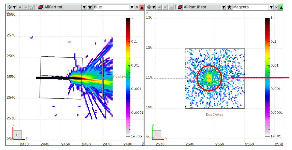
The electron beam does not hit the center of the Image Plate
