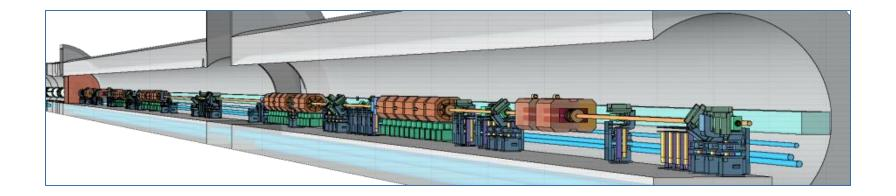
Instead of defining every replicated region (and their interior complexity) explicitly, one may define a prototype region and then use FLUKA's LATTICE capabilities to replicate it as many times as needed elsewhere in the geometry
