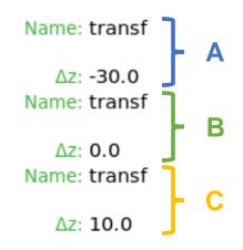
**Note:** if a transformation R consists of 3 rototranslations A, B and C applied in this order, then R = CBA and the inverse transformation is  $R^{-1} = A^{-1}B^{-1}C^{-1}$
