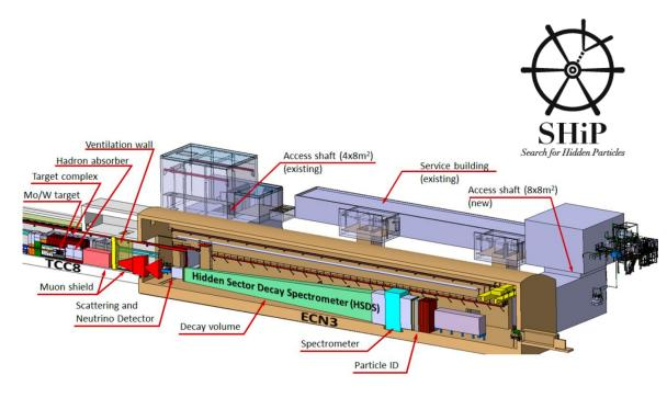
Significant opportunities for industrial return from CERN to the UK: Aim to build large systems of magnets that are essential to sweep out beaminduced muon backgrounds in the UK. This muon shield will also incorporate the SHiP neutrino detector.
