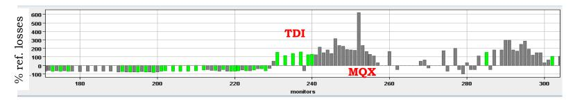
▶ Increased  $\Delta p/p$  at extraction: bunch length at extraction:  $1.5 \rightarrow 2.2$  ns → Losses on the TCDIs
