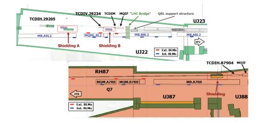
Loss reduction at downstream magnets by a factor of 2-3. Good agreement with FLUKA simulations: factor 4 predicted
