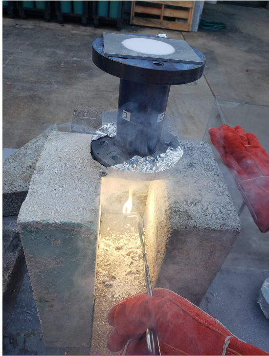
MgO layer for internal reflection
