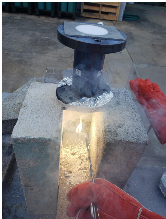
MgO layer for internal reflection
