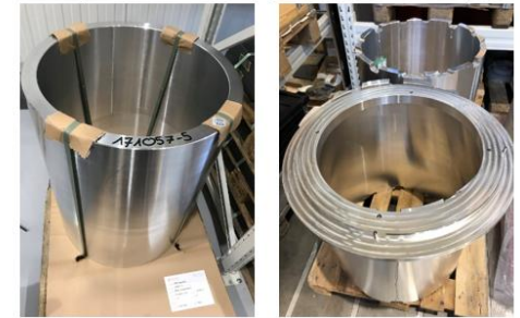
Figure 14: Al shells assembly in the MQXFb cold mass
