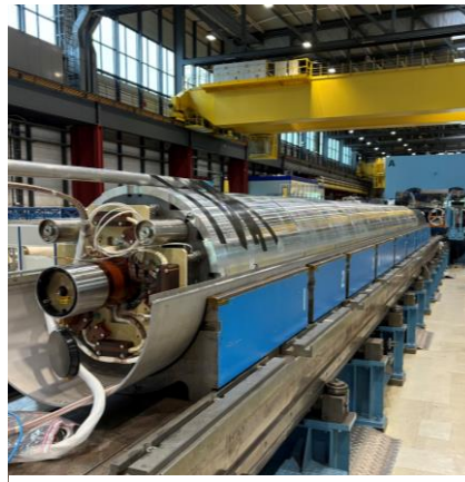
MQXFB07: preparing for welding
