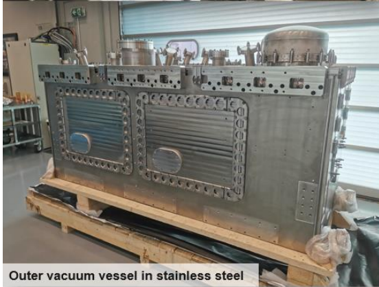
Outer vacuum vessel in stainless steel
