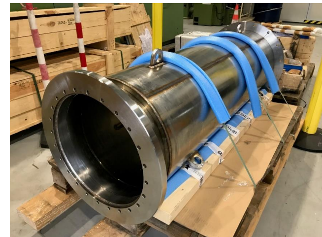
Cryocooler Test Chamber
