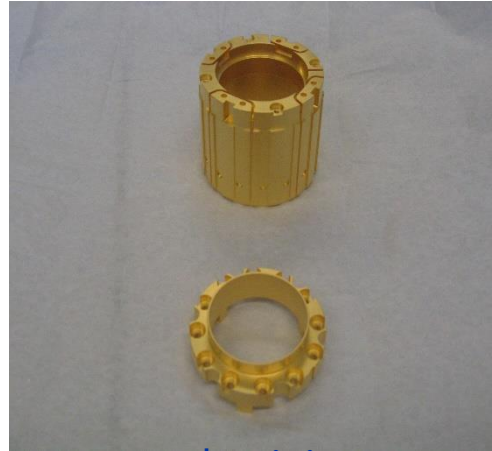
Magnets aluminium parts + gold coating
