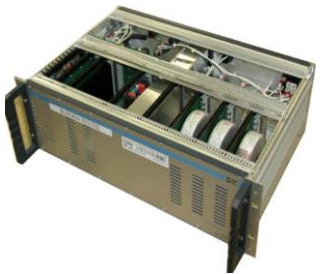
DCCT electronics: provides a voltage signal, which is then digitized by an ADC
