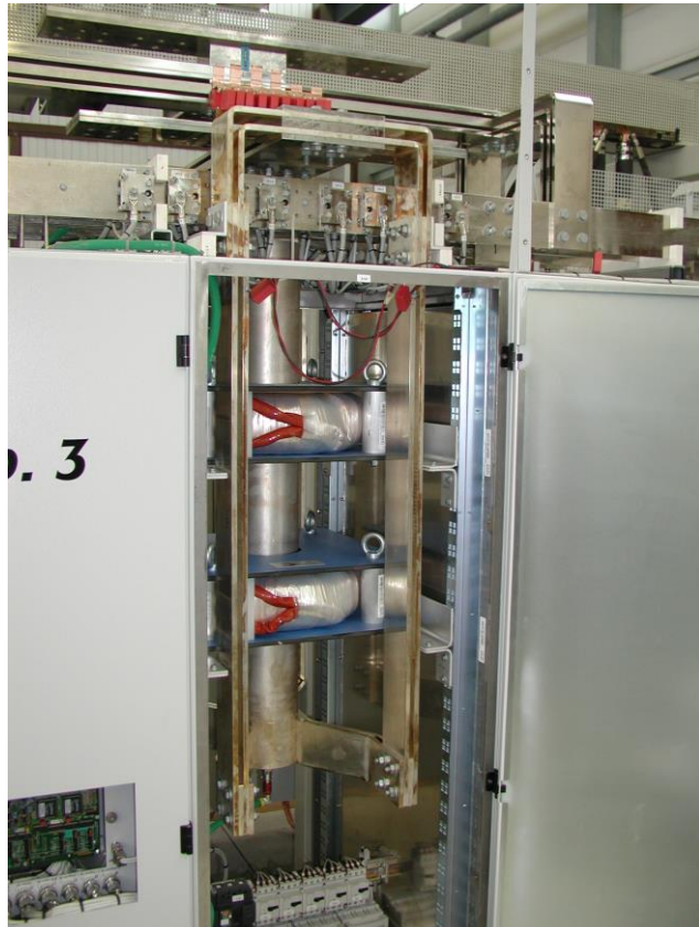
LHC DCCT 13kA magnetic head: equipped with extra winding for calibration
