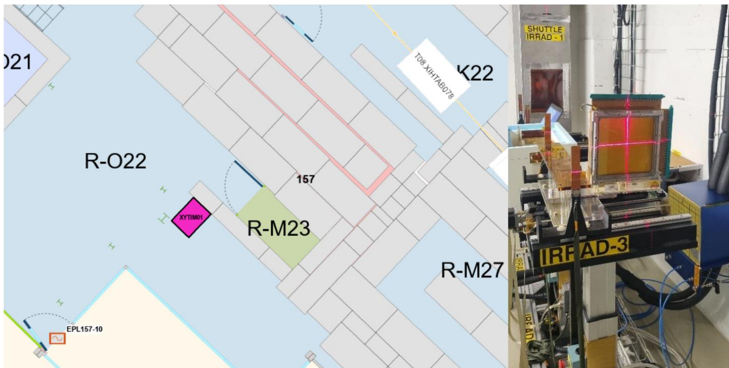
Figure 3: Location of the new MWPC (T08.XIHTAB078) and of its control electronics (XYTIM01 rack) on the left-hand side. On the right-hand side, picture of the prototype for its mechanical support on IRRAD3.
