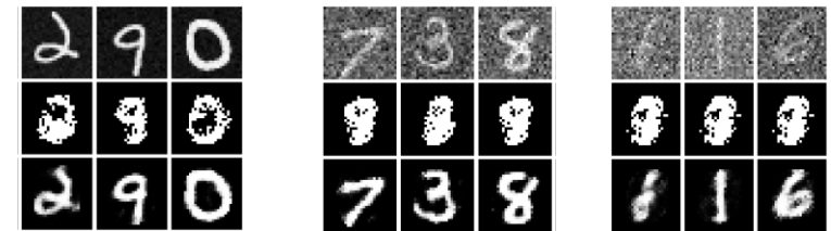
Denoising results on MNIST data (Panels: High, Medium, Low SNR) Top: Noisy data, Middle: Denoising without CN regularization, Bottom: with CN regularization
