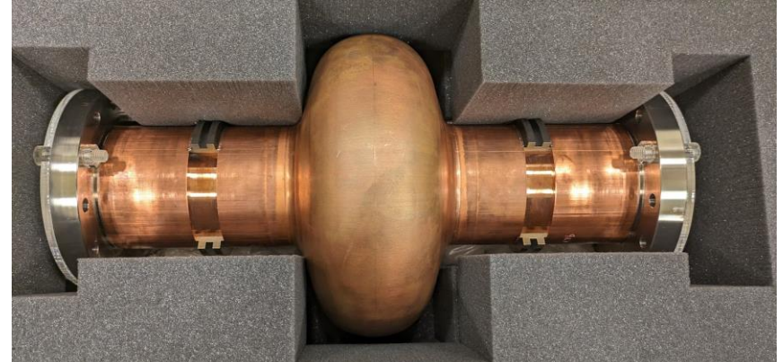
Successful 1.3 GHz hydroforming (KEK Collaboration)
