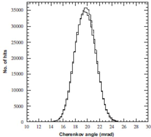
Fig. 12. Reconstructed Cherenkov angle for data (solid line) and MC simulation (dashed line) for HPD C1. There is one entry per photoelectron hit.
