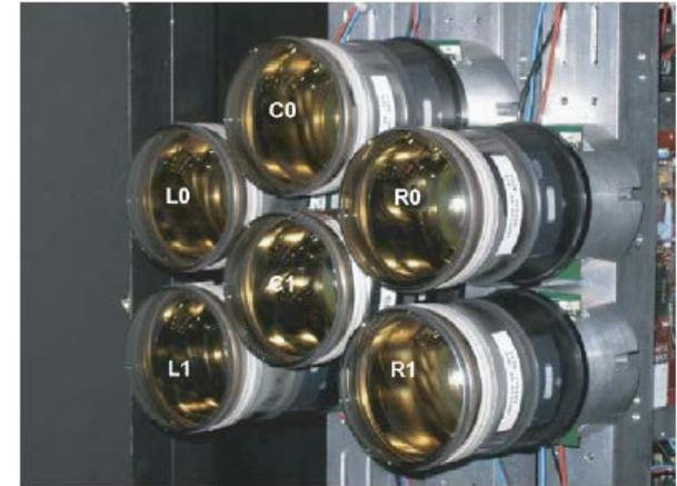
HPDs mounted in columns on two testbeams
