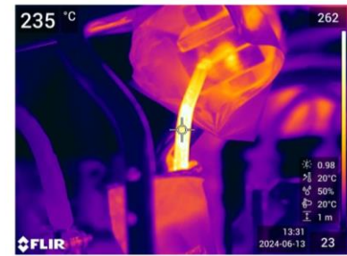
3) temperature measurements of the hottest part of the wire
