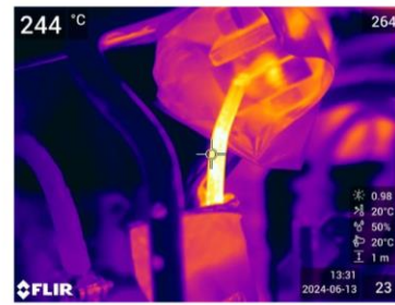
3) temperature measurements of the hottest part of the wire
