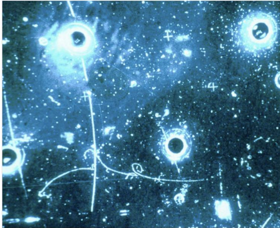
The first example of a single-electron neutral current. An incoming antineutrino knocks an electron forwards (towards the left), creating a characteristic electronic shower with electron-positron pairs (Image: Gargamelle/CERN)
