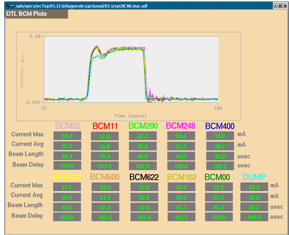
Beam pulse propagation from RFQ output to linac dump
