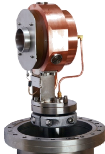
Test @GANIL -Faraday cup -Residual ionisation gas detector
