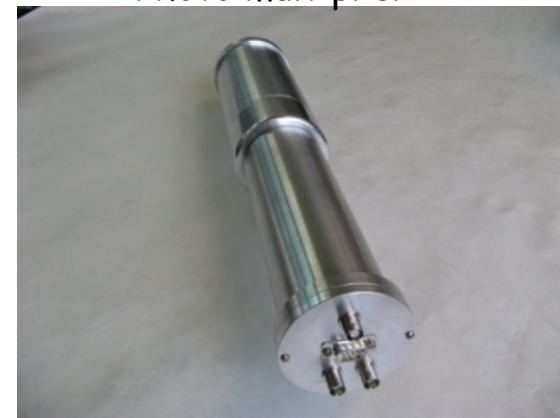
Location: 1m from beam pipe Response time E_B > 5\text{Mev} : 10 \mu\text{s} (« high » beam losses ) Spatial resolution : 1m
