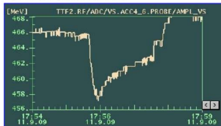
Amplitude drift of vector-sum in ACC456 for 10 deg. C temperature change of downconverter Temperature sensitivity of downconverter for amplitude is approximately 2e-3 / deg. C Temperature change just before 17:56
