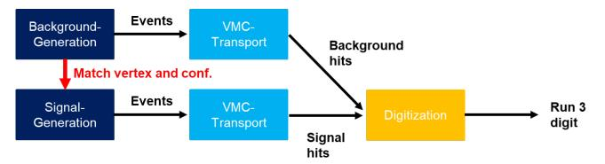
ALICE can leverage embedding techniques, i.e. generating TPC pile up events, to accelerate simulation processes, early benchmark on test machine:
