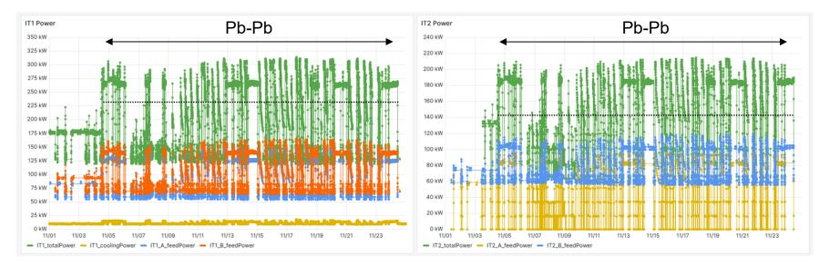
Average power consumption of 380 kW during Pb-Pb at ~50 kHz
