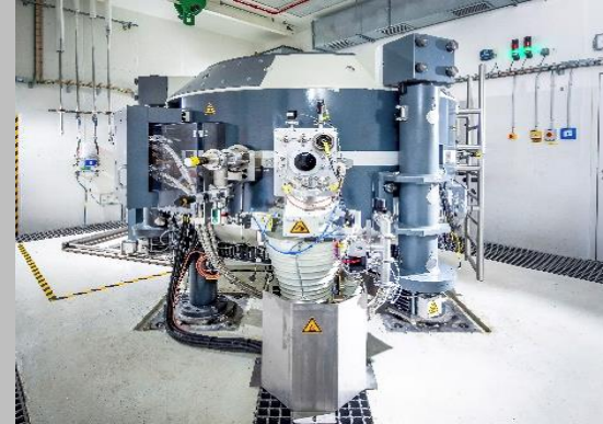
CYCLOTRON S2C2< (ProteusOne) 200 kW => ~40 kW
