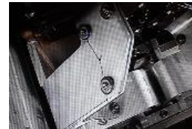
Horn stripline fatigue failure (FNAL)
