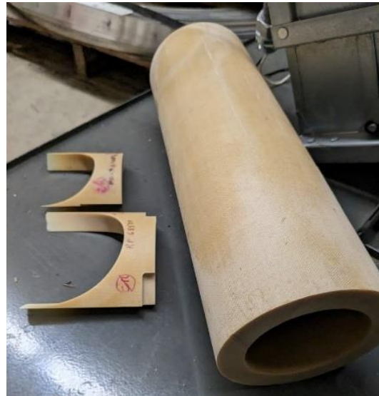
LHC MQXA inner triplet magnet endspacers made of EP GC3 (also known as G11-CR) (a) from KEK and (b) from FNAL.
