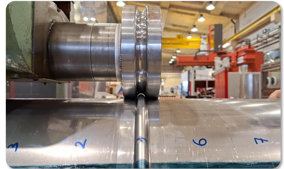
Annular corrugation performed at CERN
