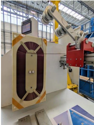
ESC Coil (Quench induction coil for SMC Magnet)
