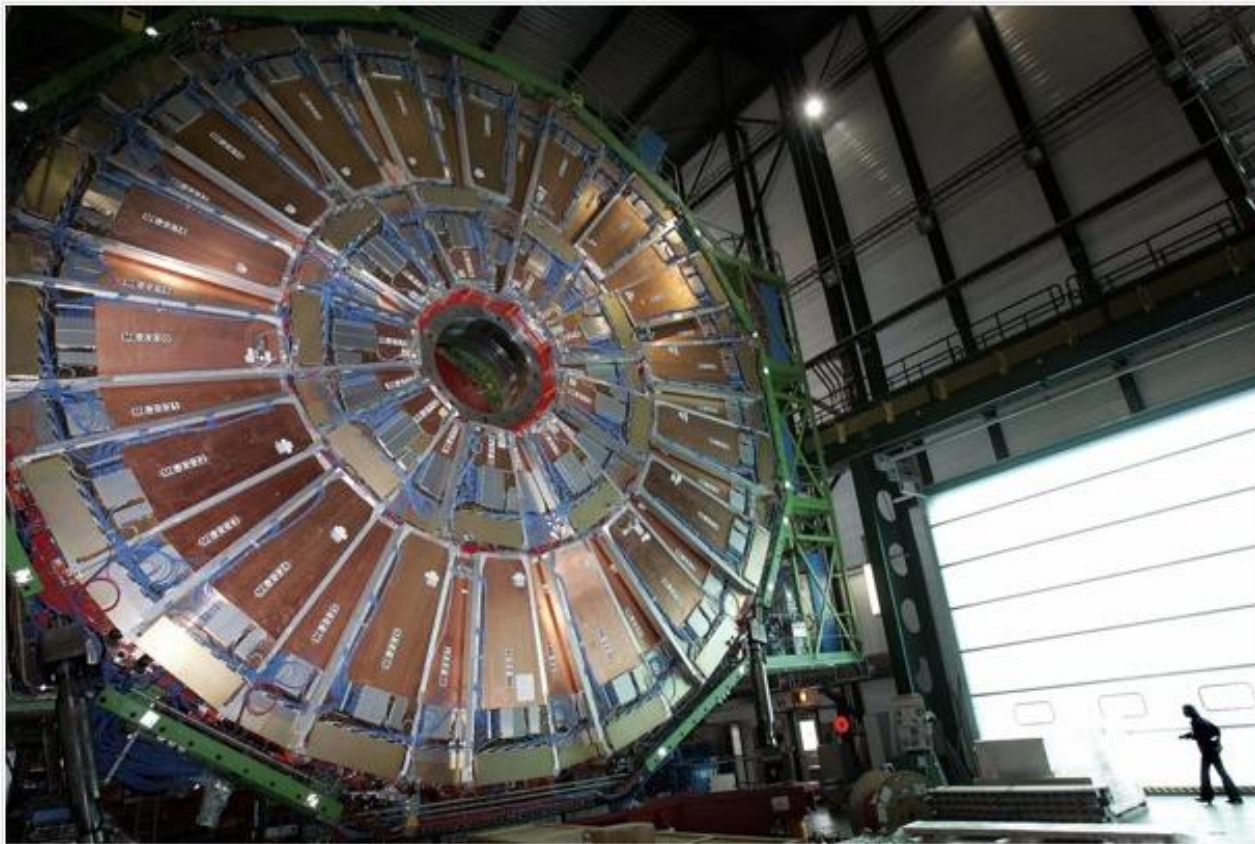
Fabrice Coffrini/Agence France-Presse via Getty Images - A superconducting solenoid magnet, the largest of its kind, is part of the Large Hadron Collider, which is searching for the Higgs boson.
