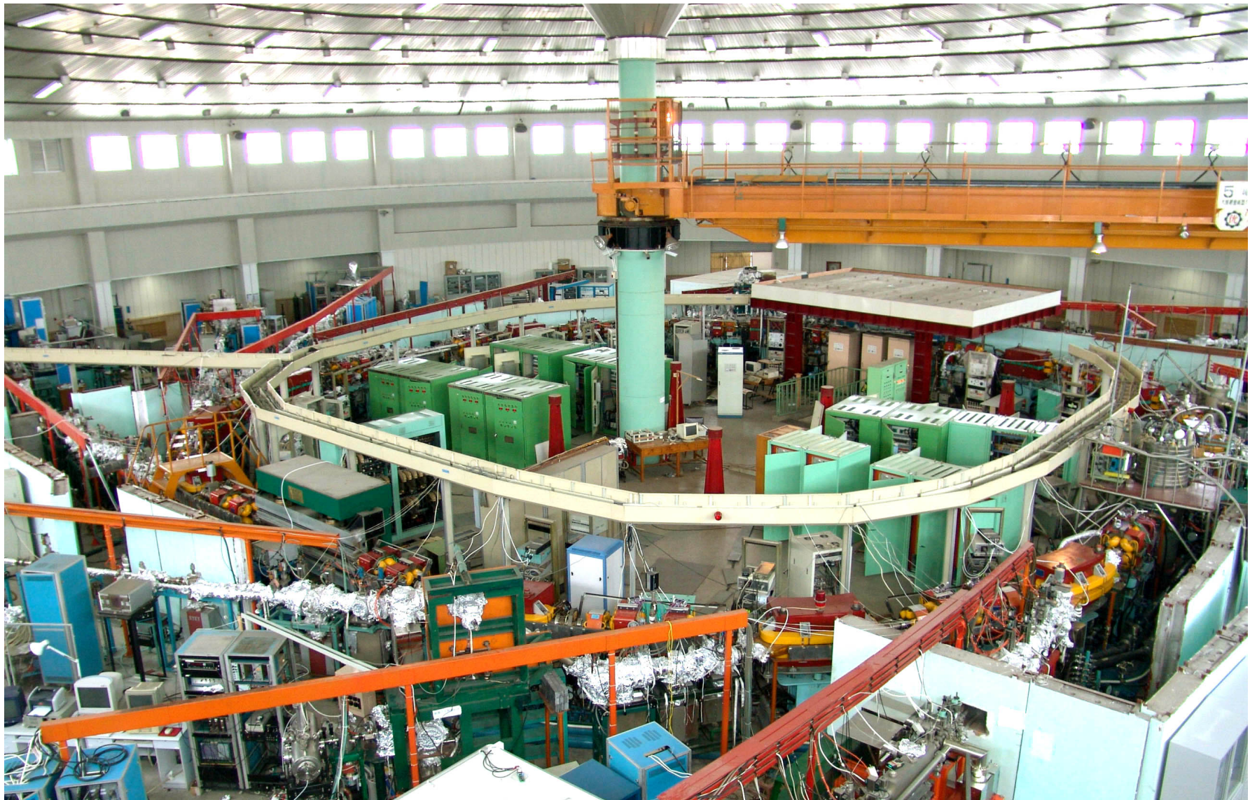
National Synchrotron Radiation Laboratory, Hefei; 0.8 GeV, 66.13 meters
