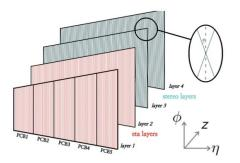
Second coordinate (**\$**) is extracted using MM stereo strips All the known B-field effects are applied
