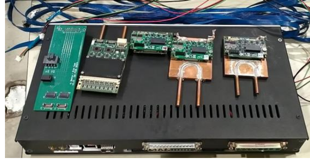
AMBER TIGER-based readout chain:
