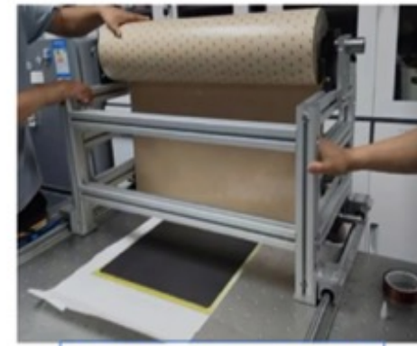
Applying insulation film
