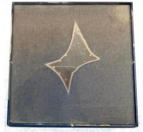
CsI photocathode after air exposure
