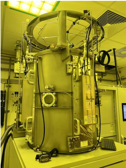
Pulsed DC magnetron vacuum deposition machine
