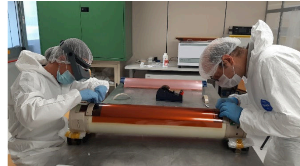
The final roof-tile is coupled to the anode support
