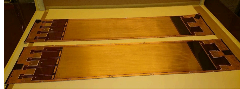
The flexible \mu -RWELL PCBs produced at CERN-EP-DT MPT Workshop. Each foil is divided in four HV sectors
