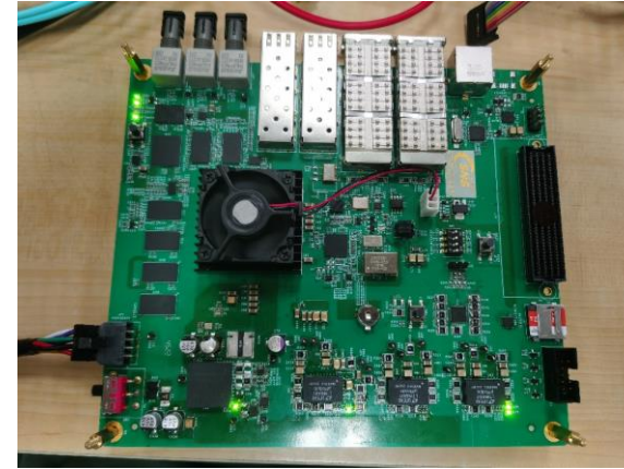
Zynq Ultrascale+ Timepix4 Readout Demonstrator
